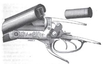
Fig. 239.—Needham's Hammerless Gun
